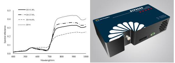
Figure 9 Original curve chart of canopy spectrum for different wheat stripe rust severity. Comprehensive use of reflectance spectral data and canopy SIF data can improve the monitoring accuracy of wheat stripe rust severity. On the right is the SIF detector produced by Optosky.
