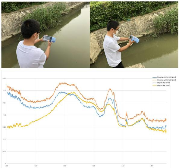
Figure 5 Application of Fieldspec hyperspectral analyzer in analyzing lake water color.
