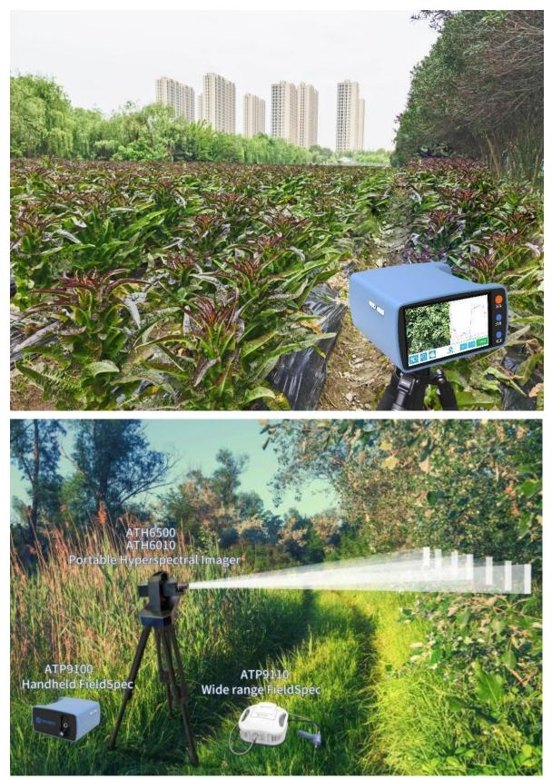
Figure 1 The cooperative use of Fieldspec spectroradiometers and hyperspectral imager.
